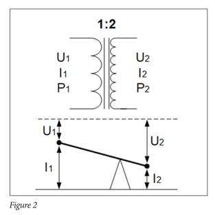
It's important to note that transformers are passive devices and cannot increase power like an amplifier. Instead, they scale voltage and current up or down as needed, to optimize a given circuit.
