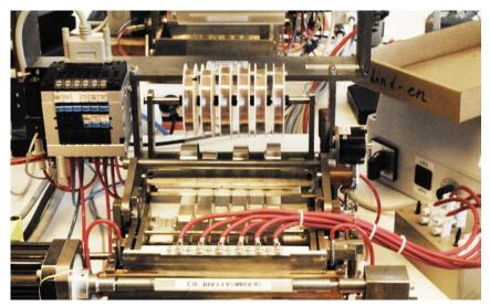
Figure 7: Awesome complexity! Front view of a Lundahl machine that inserts Faraday shields in the transformers for significantly improved CMR (Common Mode Rejection).
