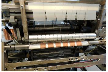
A Lundahl winding machine performing stick winding.
