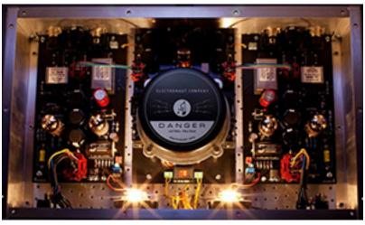
Lundahl transformers inside an Electronaut mic/instrument preamp.
