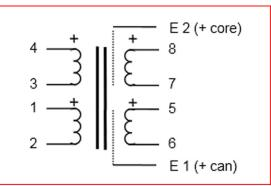
Figure 1: The schematic shows a pair of primaries (normally connected together in parallel) and two secondaries for driving two separate loads. Note the individual Faraday shields on each of the secondary windings (E 1 and E 2).
