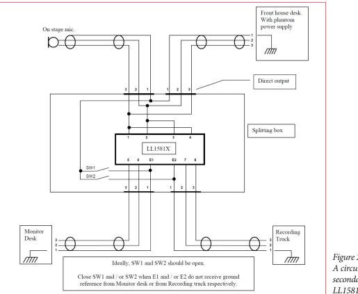
Figure 2: A circuit showing dual secondaries of a Lundahl LL1581XL splitting transformer.
